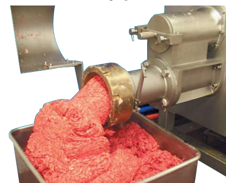
Beef Trim. 2nd Mince - 3600 kg / hr (60kg/min). Processed with 6400 66 Mixer Mincer through a 3 mm Hole Plate.
